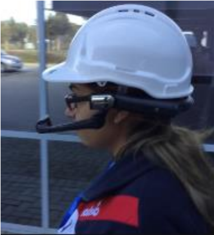
On-site team member wears the virtual support glasses & uses them to connect with a support centre SME
