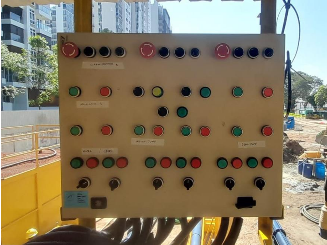
Integrated Control Panel for managing water, cement & grout batching and discharging at Grout Plant
