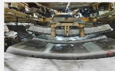
(b) Automatic Turning of Segment
