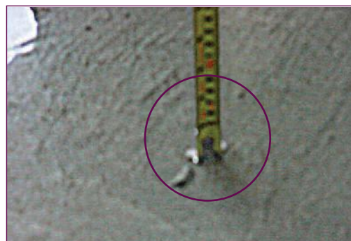
Flood to minimum 25mm for 24 hours
