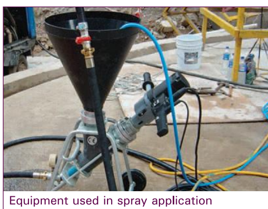
Figure 6.5: Tools for applying waterproofing membrane
