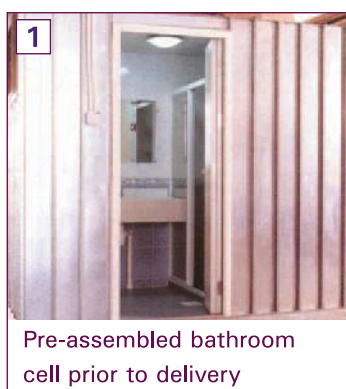
Figure 2.2: Different components of a prefabricated bathroom
