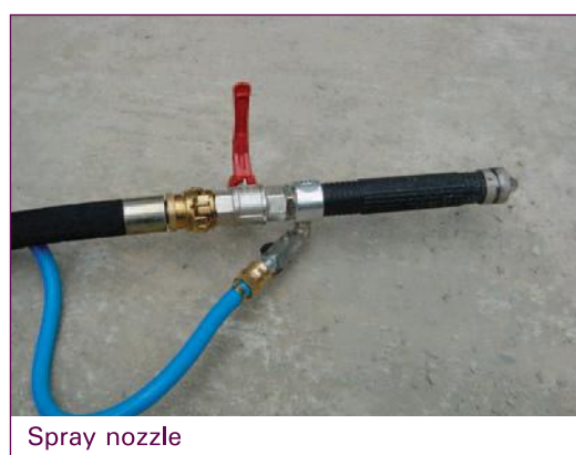
Figure 6.5: Tools for applying waterproofing membrane
