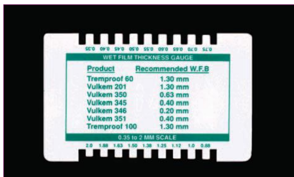
Example of a wet film thickness gauge
