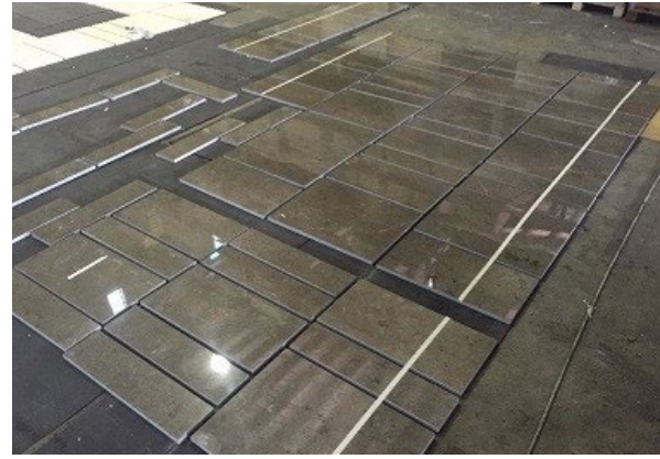
Figure 2.1.8.b. Pre-lay at factory
