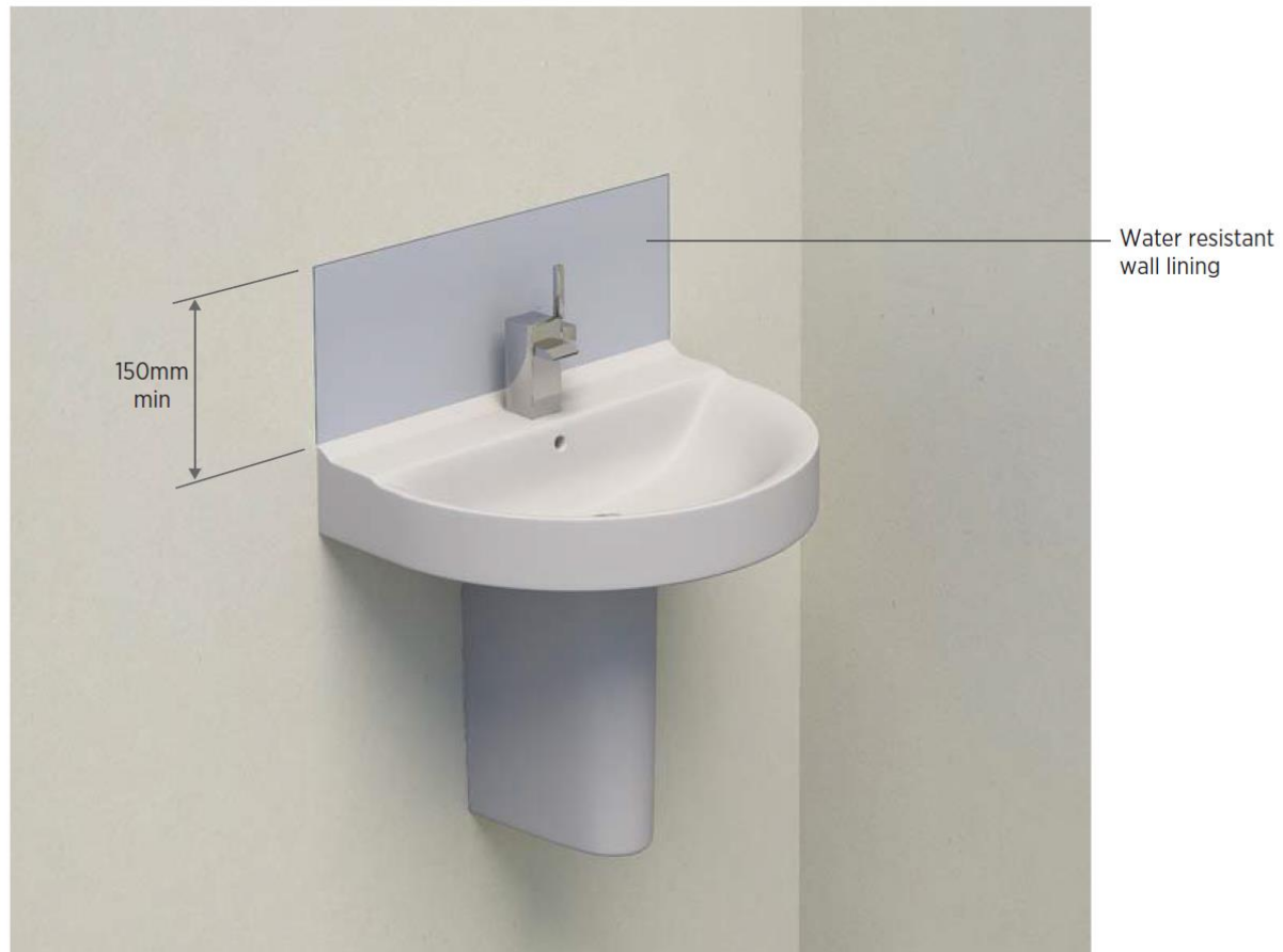
Figure 58: Waterproofing of basin
