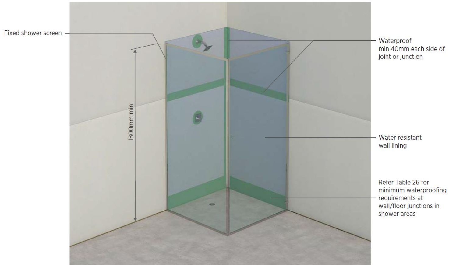
Figure 54: Waterproofing of enclosed shower
