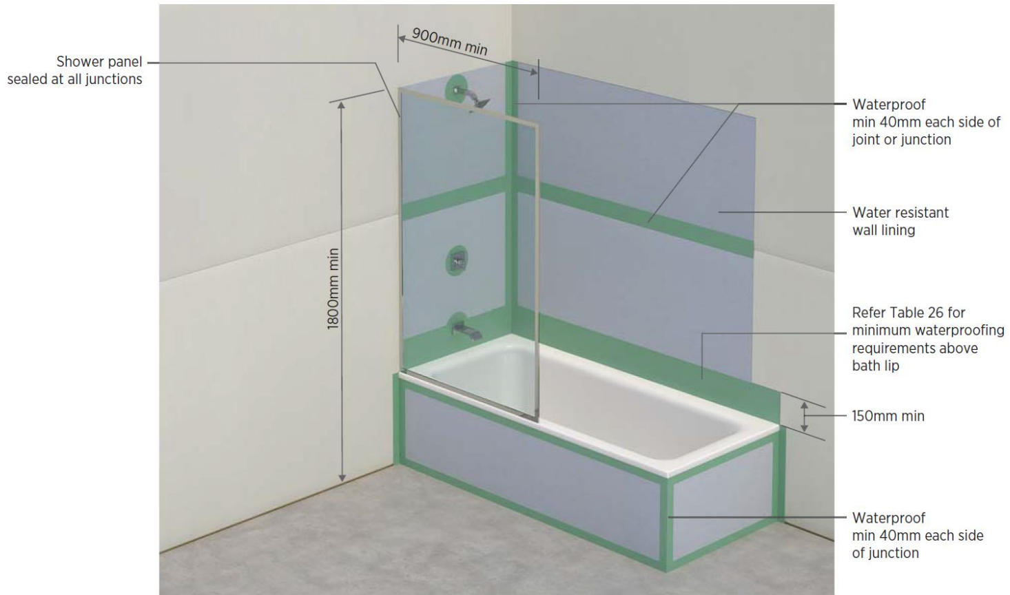
Figure 53: Waterproofing of enclosed shower over bath
