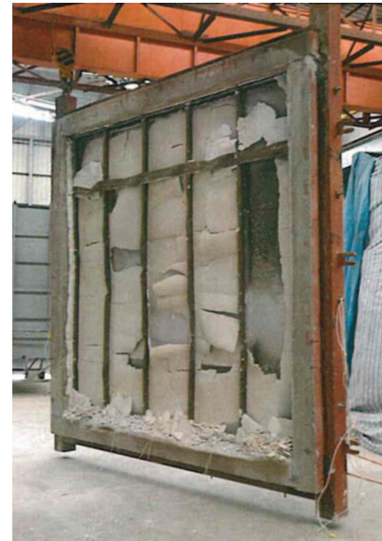
Exposed surface of the specimen after the test-1H 2 exposed layers have fallen, as well as the inner layer of the non-exposed face
