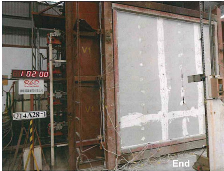
Unexposed surface of the specimen after the test – 1H
