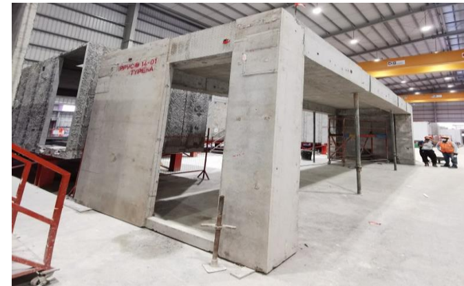
BCAA PPVC Carcass (5-sided modular shape)
