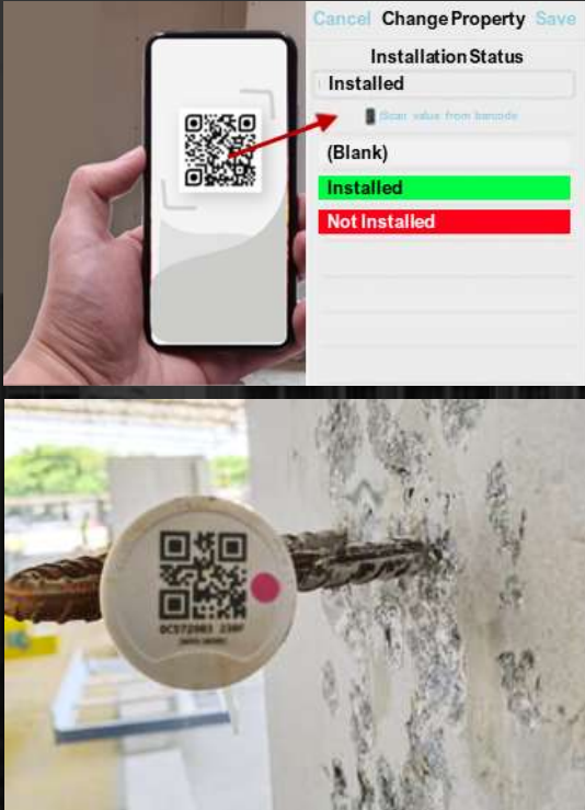
Electronic tagging systems help track the status of production and delivery of our precast components
