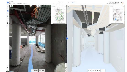
Auto Design to As-built comparison
