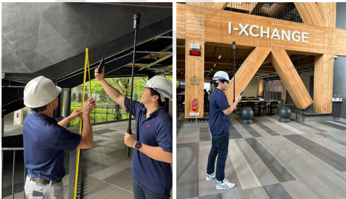
Picture 1 and 2: Virtual inspections can be done using 360 capture devices to record site findings
