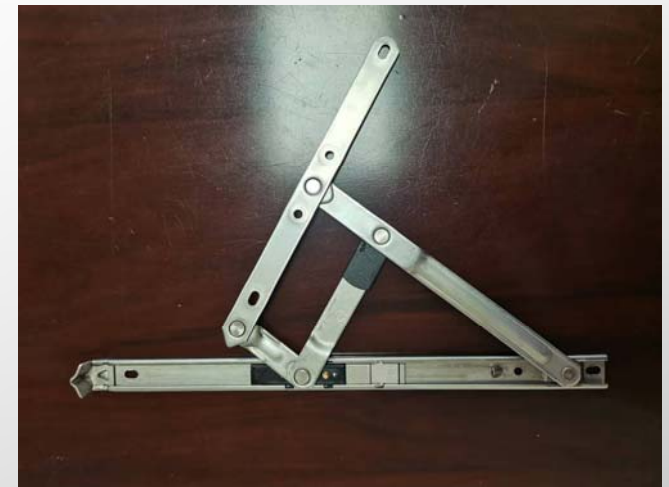
Stay with Press Button Control – Open at 30degree, lock. Press to release to full 90 degree.
