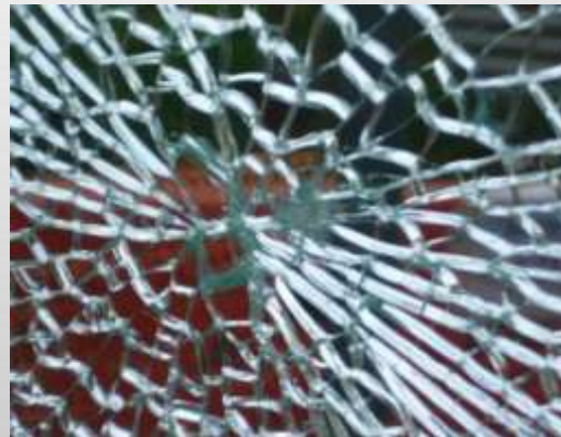
Breakage pattern – Tempered Glass.
