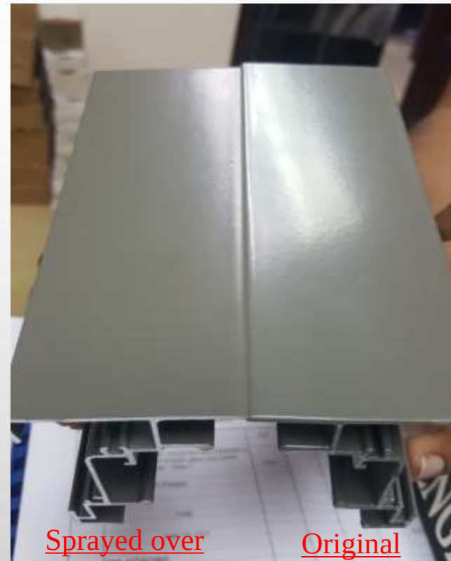
Comparison between a powder coated surface versus a spray over surface.
