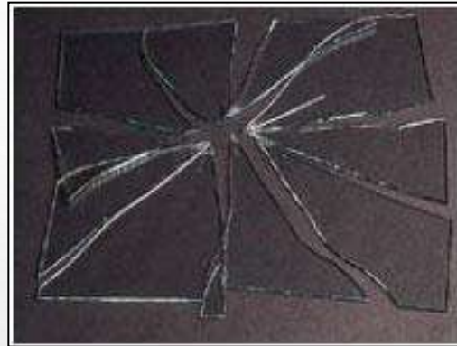
Heat Strengthened Glass - Breakage pattern.
