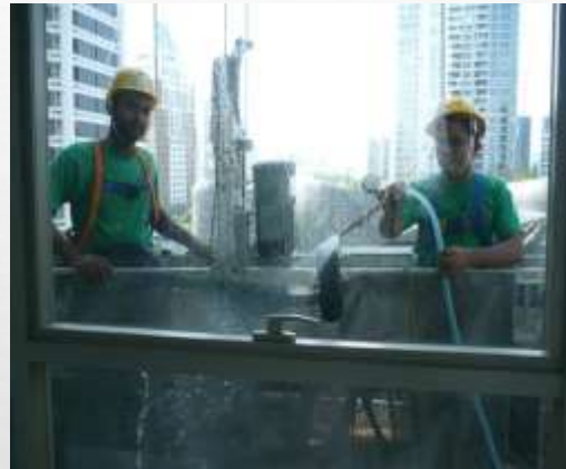
Horizontal spray – using AAMA 501.2 standard.
