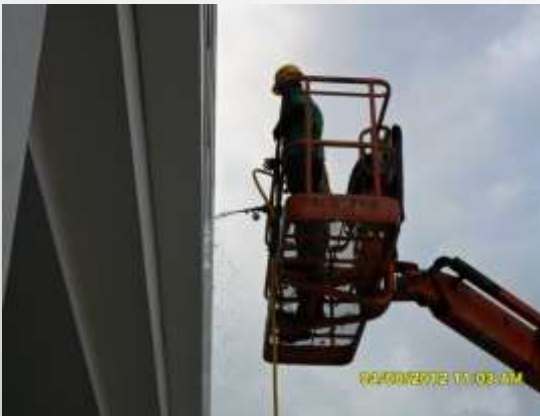
Water supply to hose – using AAMA 501.2 standard.
