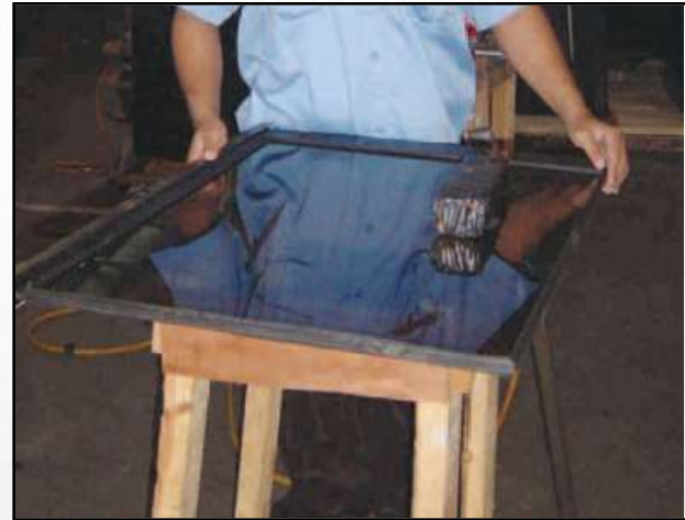
Step 2 - Gasket is inserted progressively.
