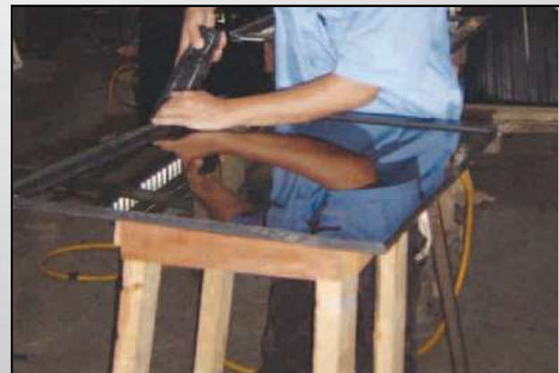
Step 4 – Full insertion of gasket to glass.
