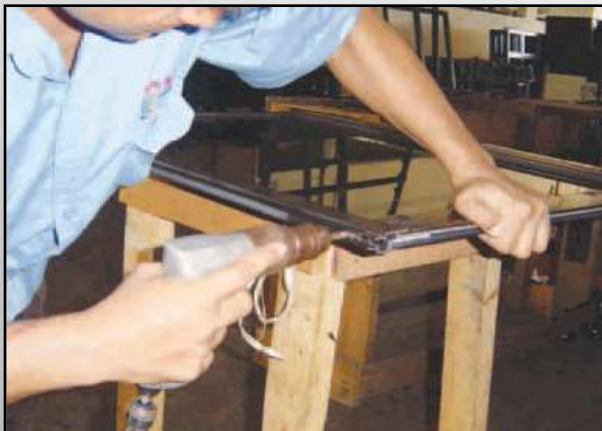
Step 3 – Assemble of outer frame.
