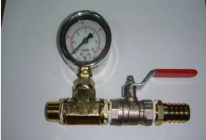
Water pressure gauge.
