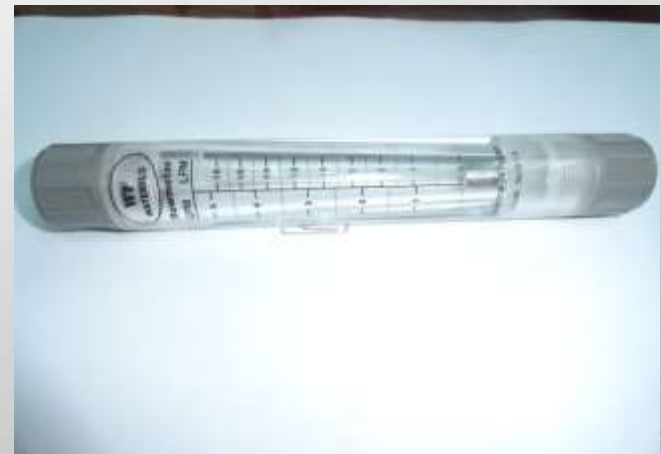
Water flow meter.
