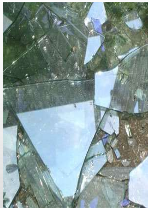
Breakage pattern – Float glass.
