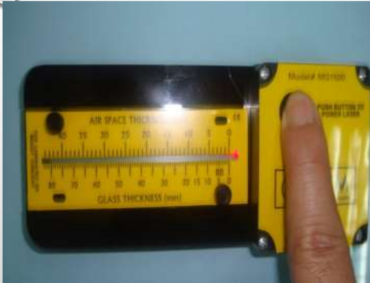
Laser gauge meter to measure glass thickness.
